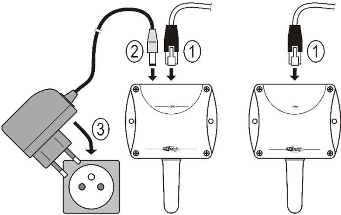
Web Sensor EPND-4S-POE and EPND-3T-POE connection (power supply adapter, Power over Ethernet):
